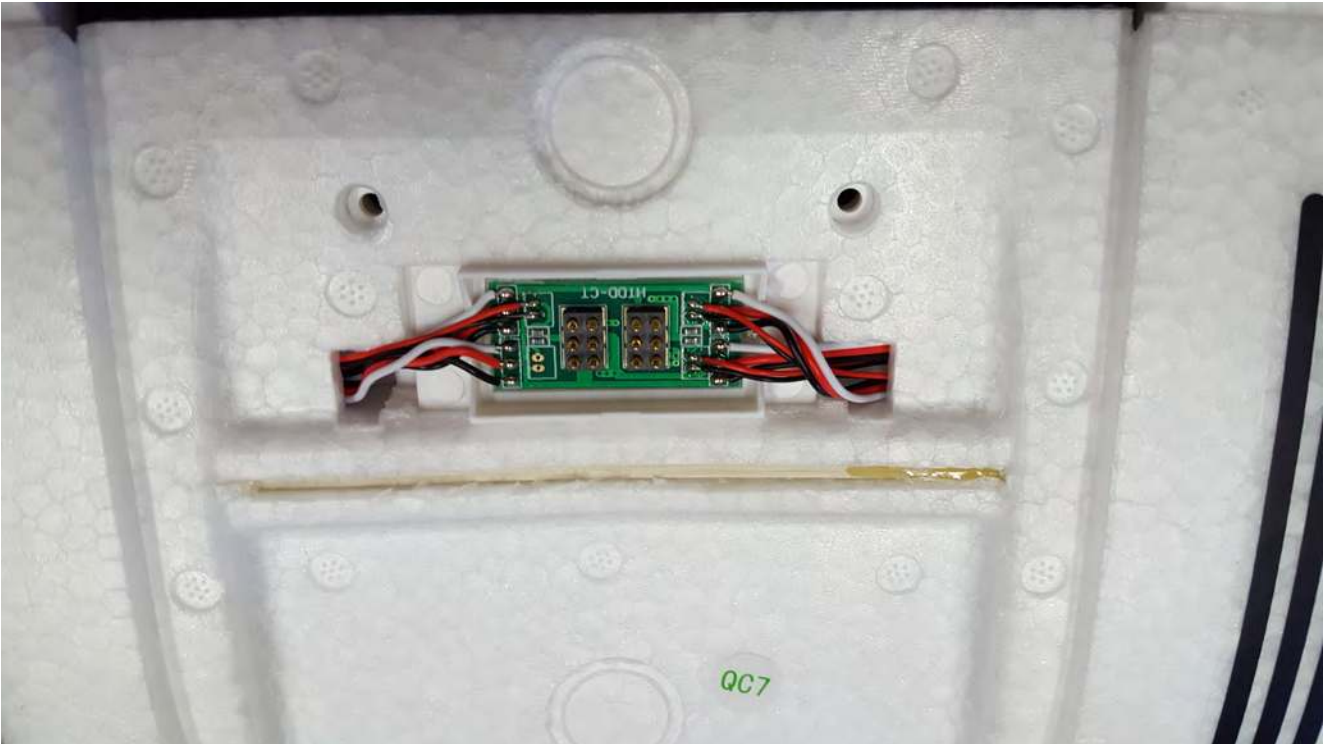
Automatic wing connection of lights, aileron and flap servos.
