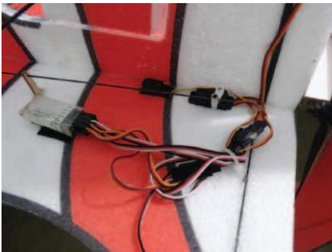
Tie all wires up with cable ties
