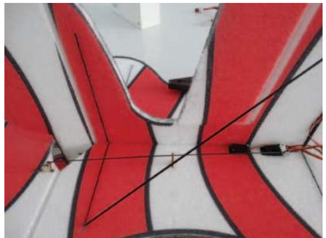
Same way to the install rudder's hinge and pull rod. Don't forgot wood strip.
