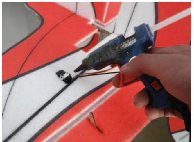
Install servo into the hole on wing using hot glue sticks.
