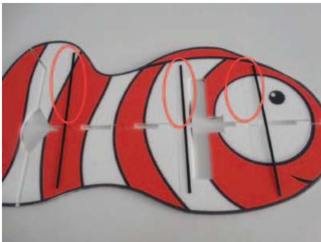
Install 3 pcs different length carbon strips on upper half vertical fuselage using foam glue. Important: don't install bottom half vertical fuselage!
