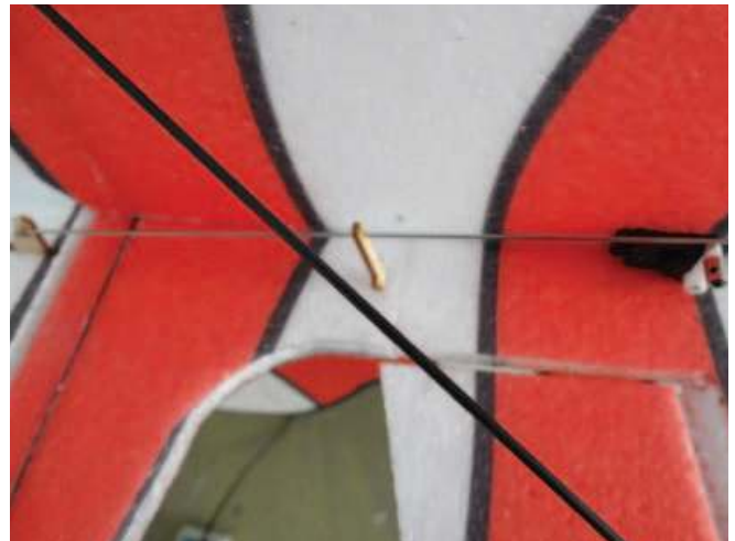
Install wood strip in the hole using No.502 glue or hot glue sticks. Notice must let pull rod through the second hole on wood strip.
