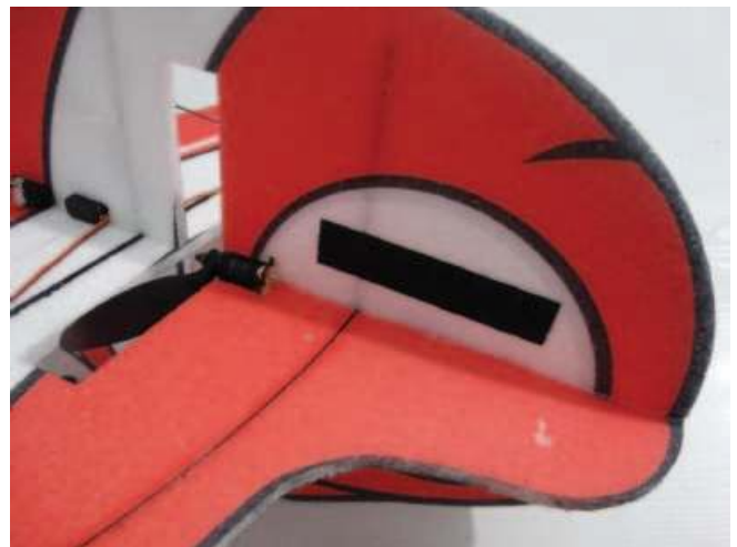
Put on hook and loop tape on fuselage using foam glue behind ESC. Then install battery.
