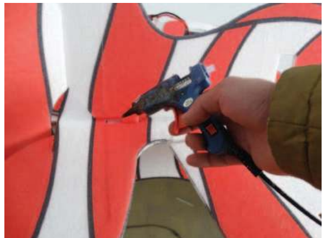
Assemble the vertical fuselage on horizontal fuselage using hot glue sticks or foam glue or No.502 glue(for indoor flying), make sure the motor mount location must be flat!
