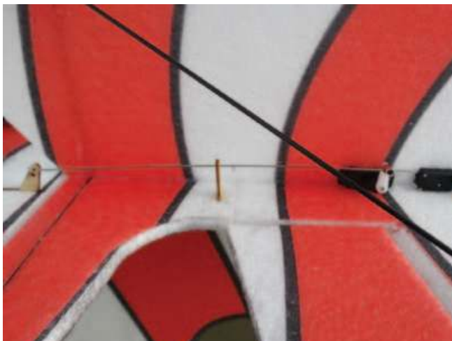
Install pull rod on servo and hinge and adjust the rod's length. Then tighten the screws.
