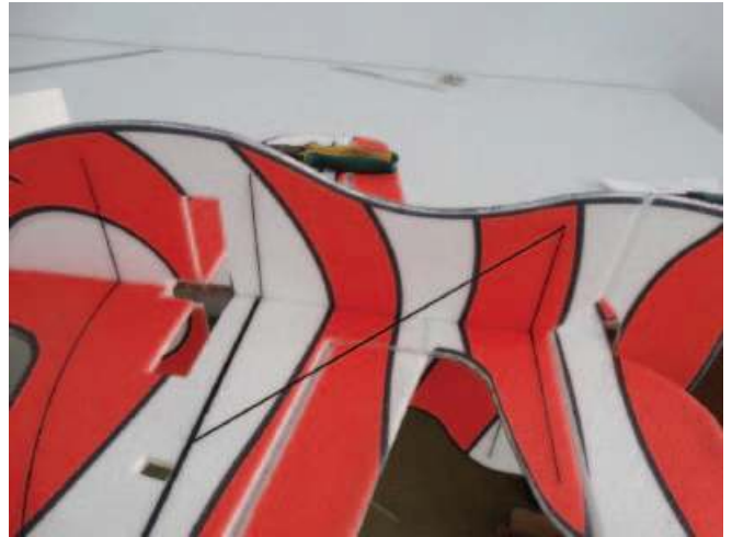
Install the 2 pcs 2mm carbon rod using No.502 glue as shown picture above. Make sure the carbon rod touch the 2pcs carbon strips.
