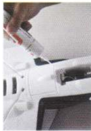
3. Glue the plastic on the bottom of fuselage.
