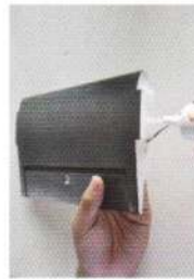
6. Fit and install the elevator. Then install the rod to the servo. And connect the elevator control line to the servo. Then apply glue to the fin.
