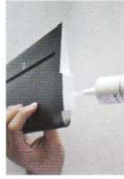
6. Fit and install the elevator. Then install the rod to the servo. And connect the elevator control line to the servo. Then apply glue to the fin.
