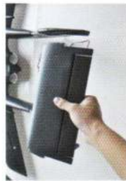
6. Fit and install the elevator. Then install the rod to the servo. And connect the elevator control line to the servo. Then apply glue to the fin.
