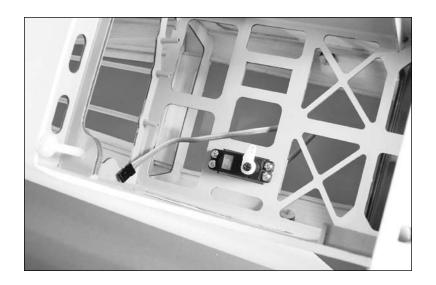
• 9. Repeat Steps 6 through 8 to install the rudder servo.
