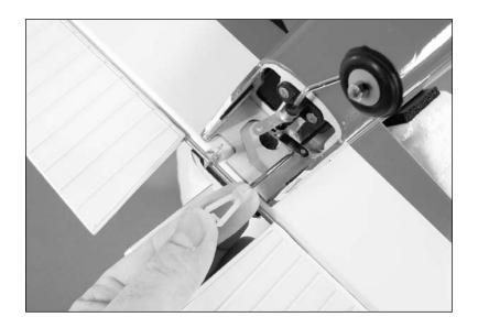
OO 12. Connect the clevis to the rudder control horn. Slide the clevis retainer over the clevis to prevent the clevis from opening and becoming disconnected from the rudder control horn.
