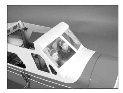
• 8. Use medium CA to glue the rear cockpit floor blocks to the sides of the fuselage slightly below the level of the center side window. There will be two blocks on each side of the fuselage as shown.
