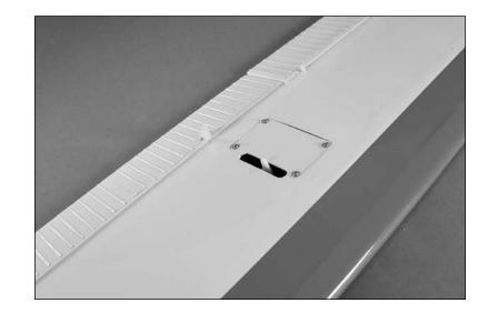
OO 11. Slide the bend of the 2<sup>3</sup>/<sub>16</sub>-inch (56mm) pushrod into the hole of the aileron servo. Secure the pushrod using the pushrod connector.
