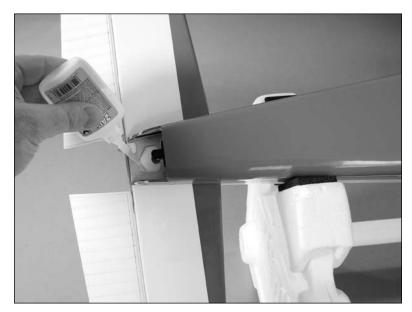
• 10. Insert the rudder control rod into the fuselage, then slide the fin into the slot in the top of the fuselage.
