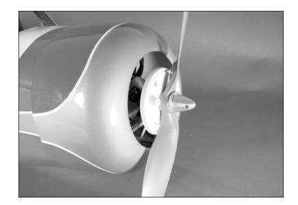
• 9. Secure the spinner cone to the backplate with the screws provided with the spinner. Use a #1 Phillips screwdriver to tighten the two screws.
