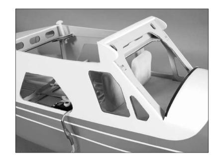
• 6. Use medium CA to secure the pilot twins to the forward cockpit floor.
