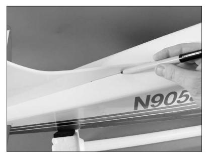
• 12. Use a sharp hobby knife to cut the covering slightly below the lines drawn. Be very careful not to cut into the underlying wood, as this will weaken the fin and cause it to fail in flight. Also trim the covering on the top of the fuselage.
