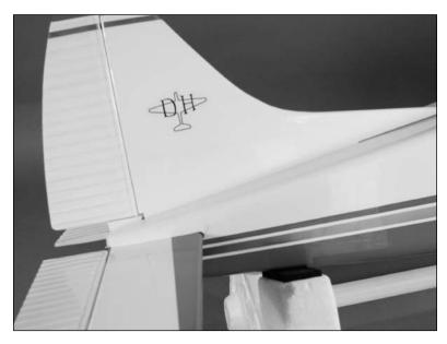
• 11. Use a felt-tipped pen to trace the outline of the fuselage onto the fin. Also trace the outline of the dorsal fin onto the top of the fuselage.
