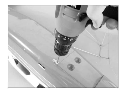
••• 4. Attach the float mount to the bottom of the fuselage using two straps, four 3mm x 12mm sheet metal screws and a #2 Phillips screwdriver.
