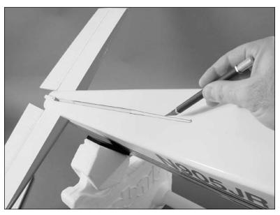
• 13. Check that the fin is square to the stabilizer. Sanding the bottom of the fin where it fits into the fuselage can correct for any alignment issues. A slight amount of material from the bottom of the fin might need to be removed for a correct fit.
