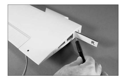
• 3. Slide the joiner into the opposite wing panel. It should slide in to slightly hide the line drawn in the previous step. If not, lightly sand the ends of the joiner until it fits equally into both wing panels.
