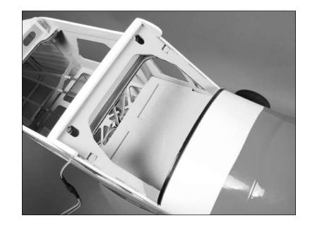
• 3. Remove the backing from the adhesive strips on the bottom of the seat backs. Attach the seat backs to the forward cockpit floor.
