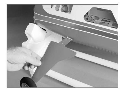
2. Secure the left half of the landing gear using two
