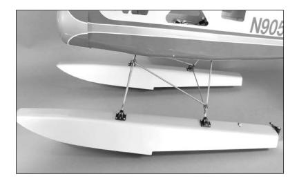
• 7. Drill a 1/8-inch (3mm) hole in the bottom of the fuselage near the landing gear. Route the float pushrod through the hole and into the fuselage. Use silicone adhesive to glue the pushrod tube to the fuselage. Use thin CA to glue the landing gear plugs to the fuselage at this time as well. You may also opt to use clear tape to install the landing gear plugs in the fuselage if you might change from floats to wheels from time to time.
