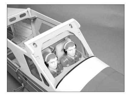
• 7. Use canopy glue to attach the front windscreen to the fuselage. Scuff the covering and windscreen where they contact each other using fine sandpaper to provide a surface for the adhesive to bond to.
