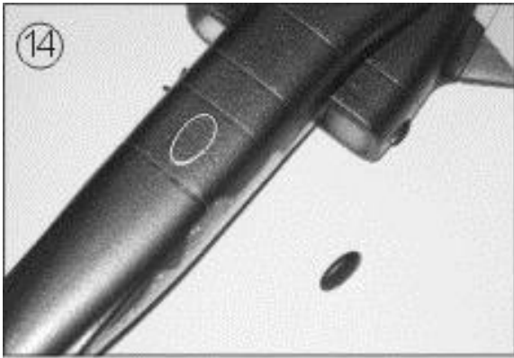
Fig. 14 - Locate the blue landing skid and apply glue to the front of the fuselage. (white mark shows the slot)
