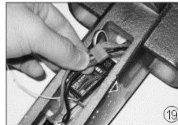
**Fig. 19** - Photo shows battery leads shown connected to the electronic speed controller.
