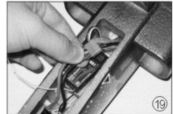
Fig. 19 - Photo shows battery leads shown connected to the electronic speed controller.
