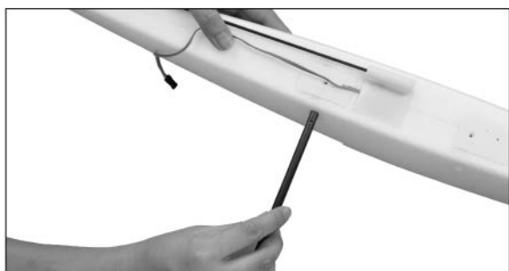
17 Connect the floats with \varnothing 8 \times 359 mm glass fibre tubes.
