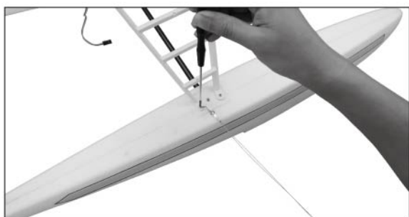
19 Fasten the brackets to the floats with PA2.5*8mm screws.
