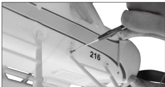
21 Fasten the float brackets to the fuselage with PA2.5*8mm screws.
