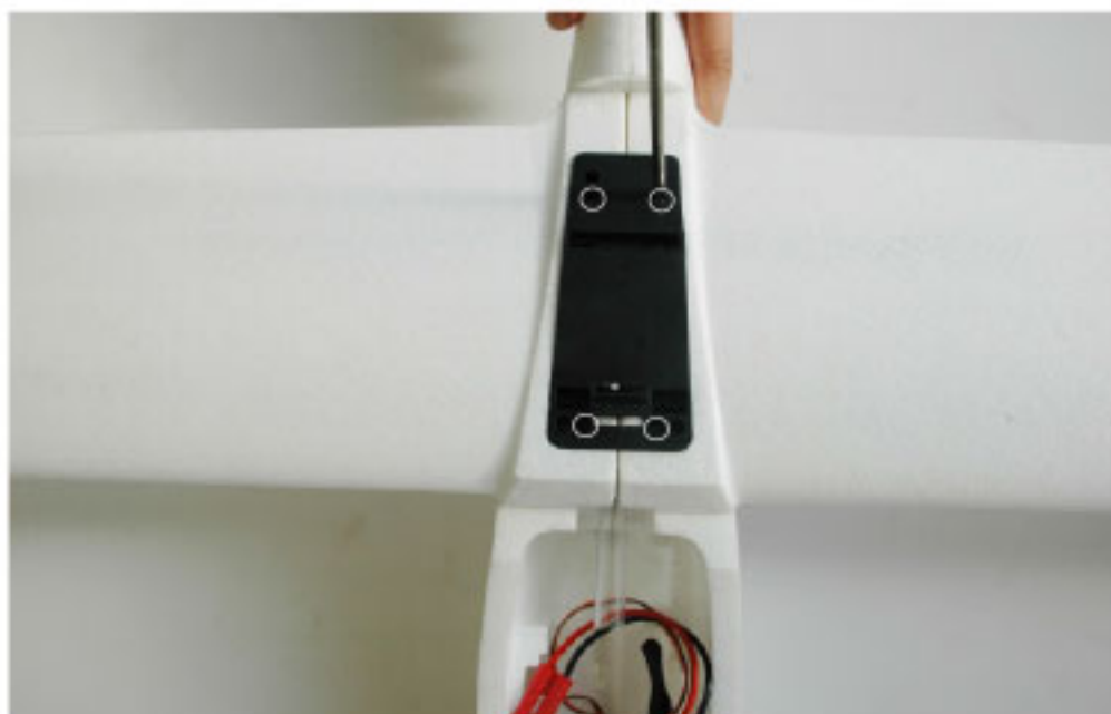
6. Secure the main wing. Screw-PM3.0*45(4PCS)
