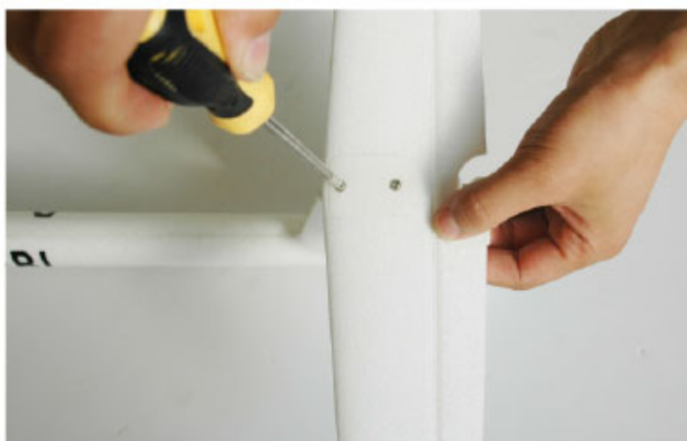
8. Install the elevator. Screw-PA3.0*20(2PCS)
