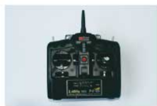
21. Turn on the transmitter before starting the power supply.
