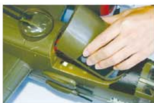
23. Install the canopy.
