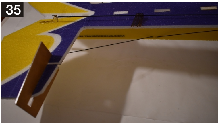
35. With the jig in place, dry fit the control rod, cut it out 1 cm before it meets the push rod stopper.
