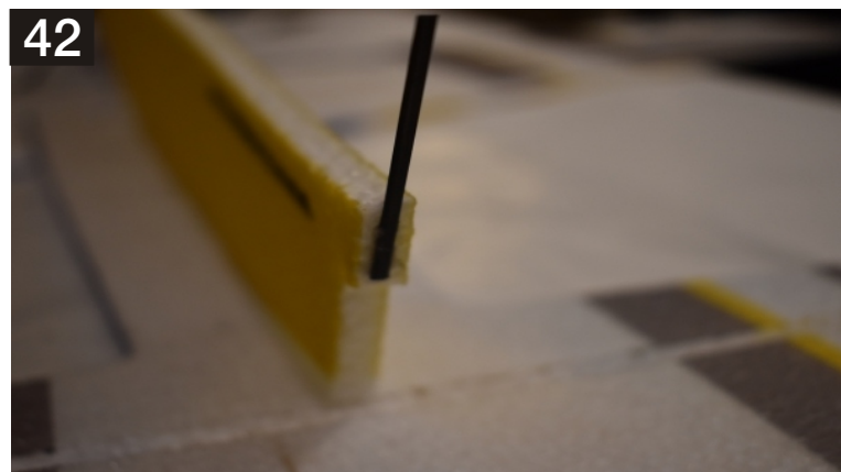
42. Locate the 60mm flat carbon strip and glue it on rear bottom part of the fuselage shown in the above image.
