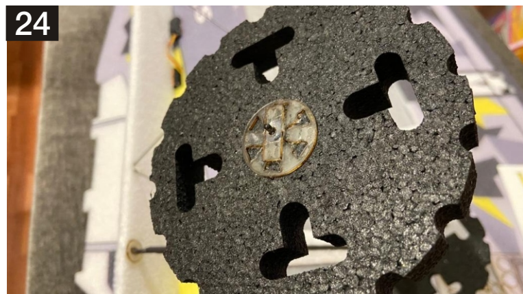
24. Install the wheel over the shaft, make sure it is spinning freely, after this slide in the wheel stopper, Put a small drop of HV CA over the shaft and wheel stopper joint.
