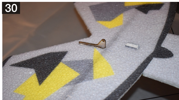
30. Glue the elevator horn shown in the image in the precut control horn slot using HV CA. Make sure it sits right to the bottom of EPP Surface.
