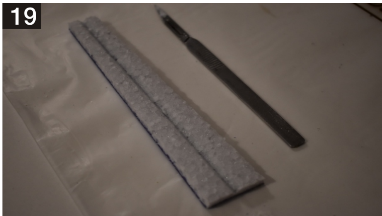
19. Locate the landing gear cover, make a V channel using the sharp knife shown in the above image. (On Non-Printed side)
