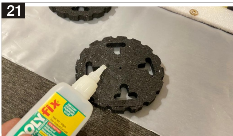
21. Spread a thin layer of HV CA over the supplied HD EPP Wheels.
