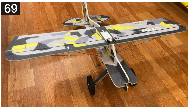
69. Here is how it will look after all the bracing is done.
