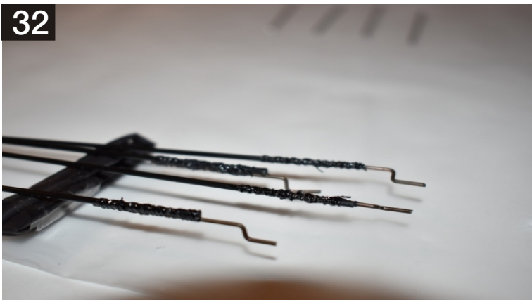
32. 47. Install the Z Bends on one side of all 4 control rods using the thread and thin CA.
