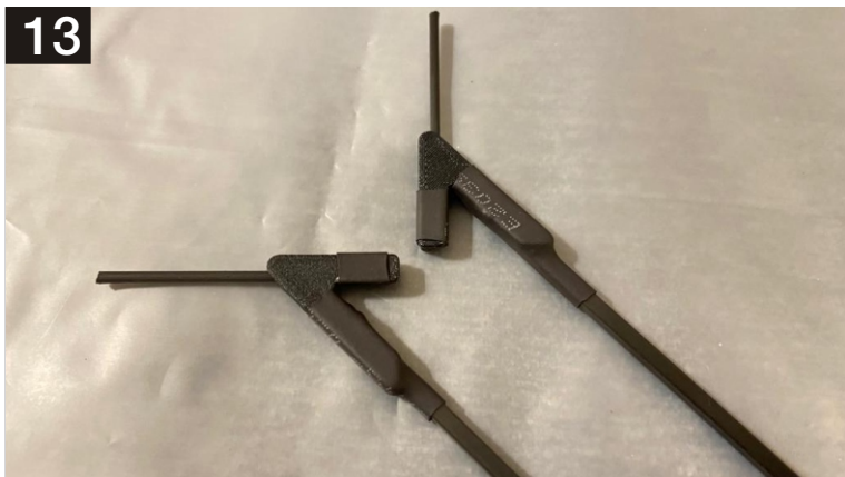
13. Here the supplied (3mm dia 225mm) tube and (2mm dia 50mm) metal wire wheel shaft are glued and heat shrunk on the wheel bracket.
