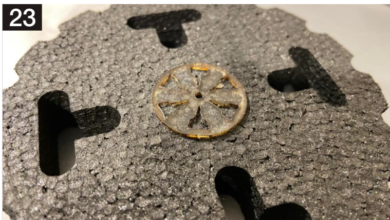
23. Glue the center rim over the wheels with center hole aligned using HV CA (Do it for both the sides of wheels).
