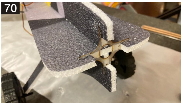
70. Install the motor mount using HV CA, Place adhesive on the inside of the mount covering every spot, then place again on the front of the fuselage making sure everything is flush and lined up correctly.
